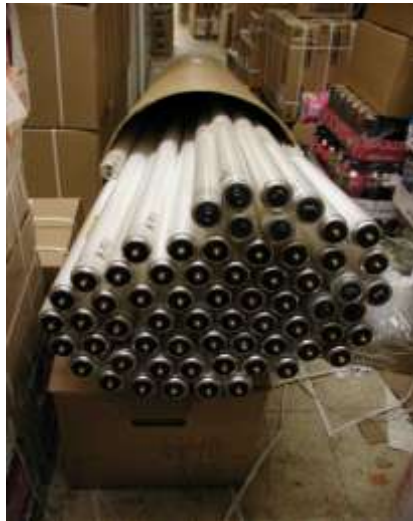
8ft, T-12 lamps prepared for recycling.
