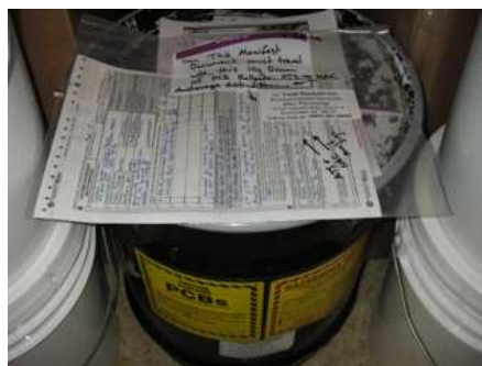
DOT approved shipping manifests and haz-mat container of PCB ballasts ready for shipment
