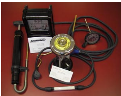
Components of a Bacharach Flu Gas Analyzing Kit used in boiler efficiency training and left with capable maint staff in their villages.
