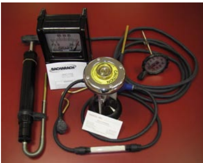
Components of a Bacharach Flu Gas Analyzing Kit used in boiler efficiency training and left with capable maint staff in their villages.
