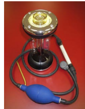
Flu gas analyzer measures levels of unburned carbon in combustion gases
