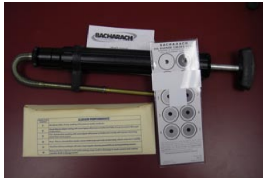
Smoke-test kit for analyzing flue gases for boiler efficiency
