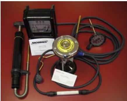
Components of a Bacharach Flu Gas Analyzing Kit used in boiler efficiency training and left with capable maint staff
