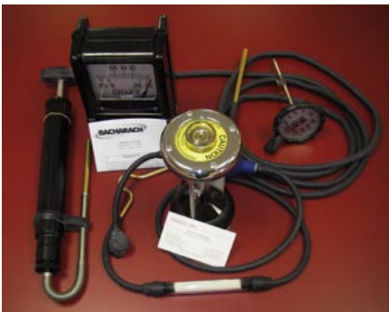
Components of a Bacharach Flu Gas Analyzing Kit used in boiler efficiency training and left with capable maint staff
