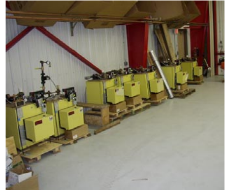
New Energy Kinetics System 2000 Low-Mass Boilers – awaiting installation in BSSD buildings
